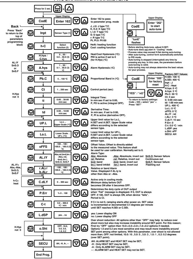
(1) When sensor type is changed, Up.L, Lo.L, H.Set, A.Set, H.hys, A.hys, r.Alr, b.Alr, oFFs may be set to a new value automatically, according to the selected sensor.
